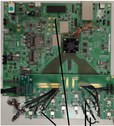
AMD ZCU670 with Wupatec Vector Signal Transceiver firmware
